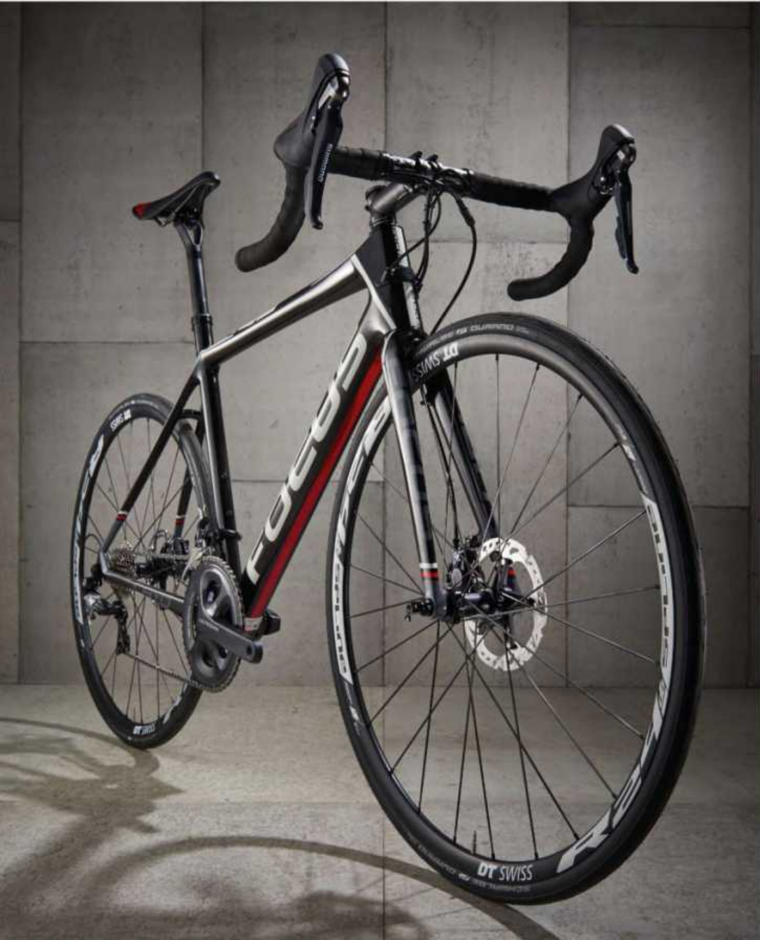
+ ↓ Below Thru-axles and hydraulic brakes form a great pairing Bottom The Focus features neat split seatpost for extra comfort
