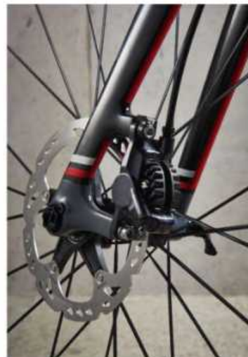
+ ↓ Below Thru-axles and hydraulic brakes form a great pairing Bottom The Focus features neat split seatpost for extra comfort
