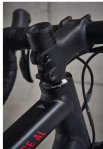
+ ↓ Below Spacers above the stem give you a bit of adjustability Bottom A shade over a grand and full Ultegra – minus chain – is great to see
